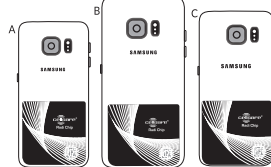
A Chip position on Samsung Galaxy S7 B Chip position on Samsung Galaxy S7 Edge C Chip position on Samsung Galaxy S8
