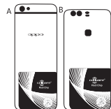
A Chip position on Oppo B Chip position on Huawei
