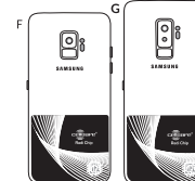
F Chip Position on Samsung S9/S10 G Chip Position on Samsung S9+/S10+
